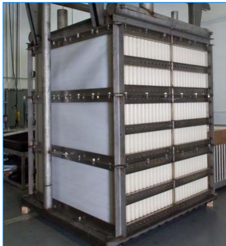
A module consists of multiple membrane plates
