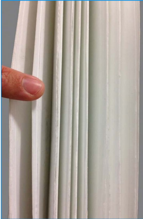
A module consists of multiple membrane plates
